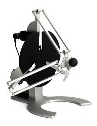
The **delta.3** is a high performance force feedback interface based on the delta manipulator. It offers 3 active degrees-of-freedom in translation and features a **larger workspace** than omega.x devices. Thanks to its unique parallel mechanical design, the **delta.3** can convey **large continuous forces** anywhere in its workspace.
