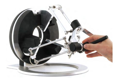
The **omega.6** is the most advanced pen-shaped force-feedback device available. Building on the omega.3 base, its design provides **perfect decoupling** of translations and rotations. The combination of **full gravity compensation** and **driftless calibration** contributes to greater user comfort and accuracy. Conceived and manufactured in Switzerland, the omega.6 is designed for demanding applications where **performance and reliability** are critical.
